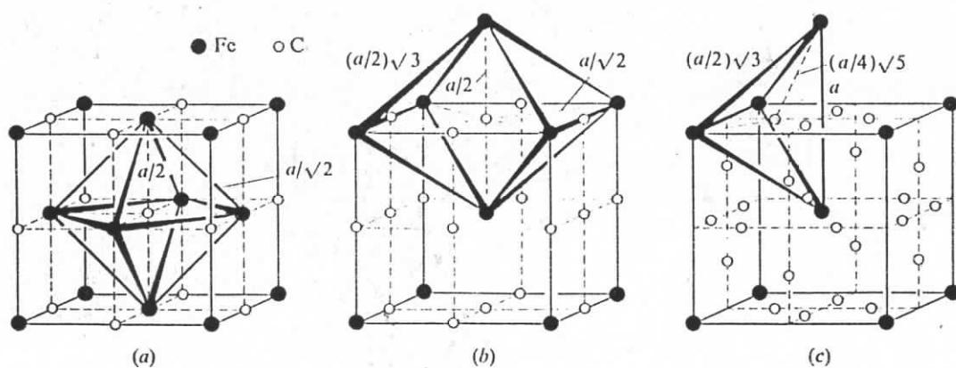
Fig. 6.7. Interstitial lattice sites for carbon in iron. (a) octahedral interstices in  $\gamma$ -(fcc) iron; (b) octahedral (c) tetrahedral interstices in  $\alpha$ -(bcc) iron.
