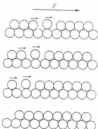
**Fig. 4.18.** The glide of a dislocation represented by a missing atom. Under the action of an external stress, the atoms around the dislocation slip to the right. The dislocation moves to the left and eventually disappears, leaving a surface step with a depth equal to one interatomic spacing.
