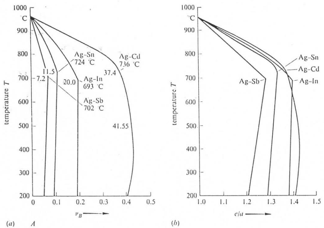
Fig. 6.18. Extent of the  $\alpha$ -phase in silver solid solutions (a) plotted against mole fraction; (b) plotted against electron concentration.
