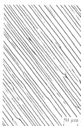
Fig. 4.12. Slip lines on an aluminium crystal (by kind permission of G. Wyon).
