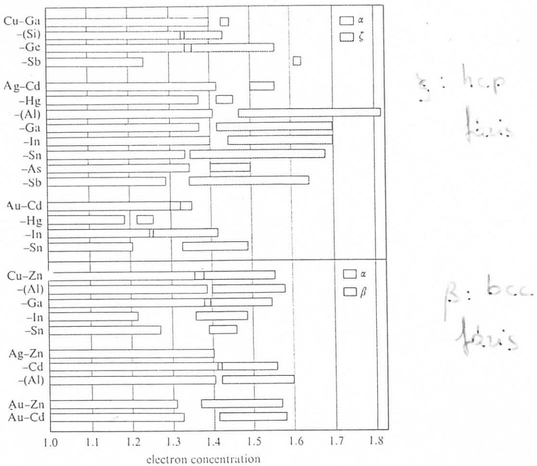
Fig. 6.19. Extent of the phases  $\alpha$  (primary solubility),  $\zeta$  and  $\beta$  for solid solutions of Cu, Ag and Au with B-metals. After [2.1].
