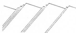
Fig. 4.13. Diagrammatic representation of slip bands resolved into groups of closely spaced slip lines.
