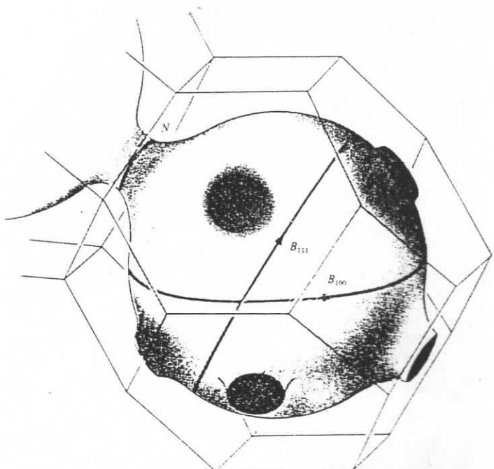
Fig. 6.22. Fermi body of copper in the first Brillouin zone with 'necks'  $N$  and 'bellies' of different circumference ( $B_{111}$  and  $B_{100}$ ) [1.1] after Dinnard
