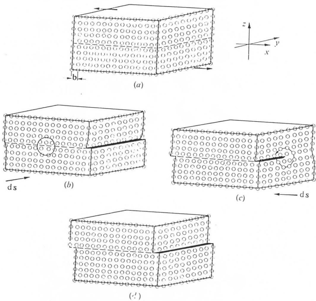
Fig. 11.1. The two possible intermediate steps in the elementary slip process in crystals (a) to (a), namely (b) the edge dislocation and (c) the screw dislocation.
