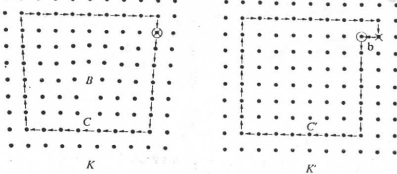
Fig. 11.3. Burgers circuit  $C$  round a 'bad' crystal region  $B$  in the crystal  $K$  and  $C'$  in the perfect crystal  $K'$  with closing vector  $b$ .
