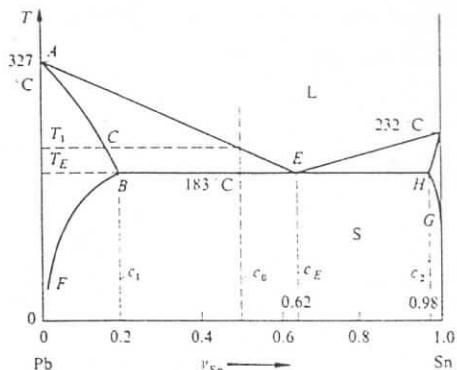
Fig. 4.13. Lead-tin phase diagram.
