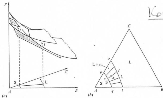
Fig. 5.22. A tangential plane construction to the free energy surfaces defines equilibrium between  $s$  and  $l$  in the ternary system (a). Isothermal section through a ternary phase diagram obtained in this way with a two-phase region ( $L+S$ ) and various conodes (b). The quantities of  $l$  and  $s$  at point  $x$  are determined by the lever rule.
