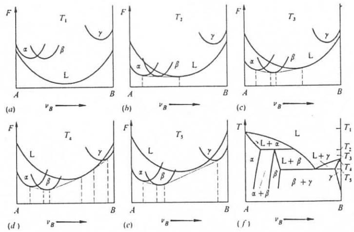
Fig. 5.19. Derivation of a phase diagram with an intermetallic compound  $\beta$  which forms peritectically.
