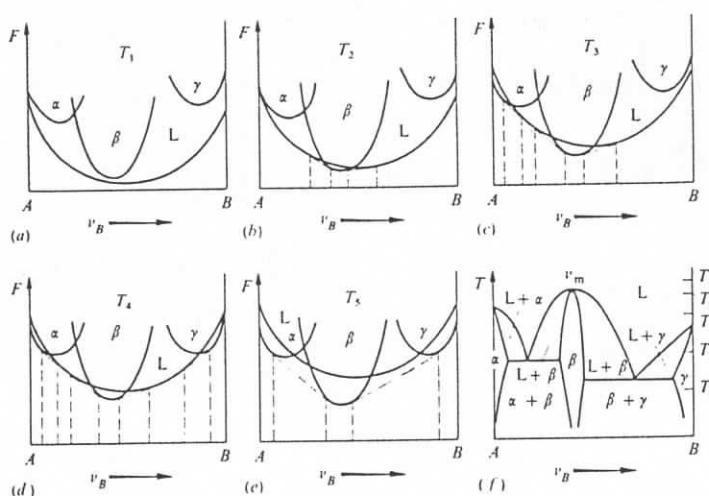
Fig. 5.18. Free energies and the phase diagram derived from them with the intermetallic compound  $\beta$ , which forms directly from the melt L.
