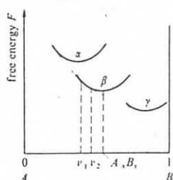
Fig. 5.17. Free energies of three phases  $\alpha$ ,  $\beta$ ,  $\gamma$ . The compound is stable between  $v_1$  and  $v_2$  but not at its stoichiometric composition  $A_xB_y$ .
