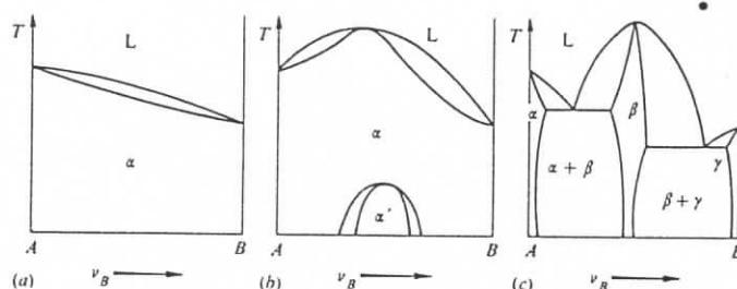
Fig. 5.16. Changes in the phase diagram from (a) to (c) with increasingly negative  $\epsilon$  or  $E^M$ .  $\beta$  is the intermetallic compound  $A_xB_y$ .
