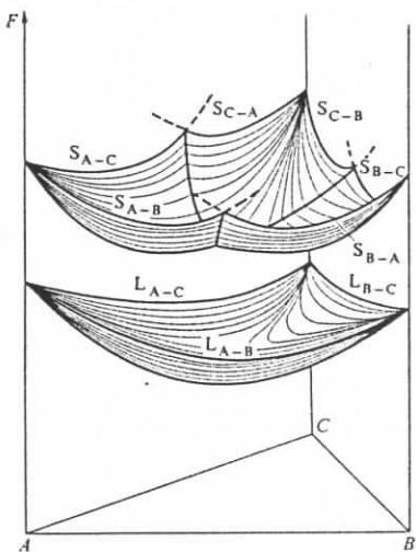
Fig. 5.21. Free energies of a liquid (L) and three solid (S) phases of a ternary system.
