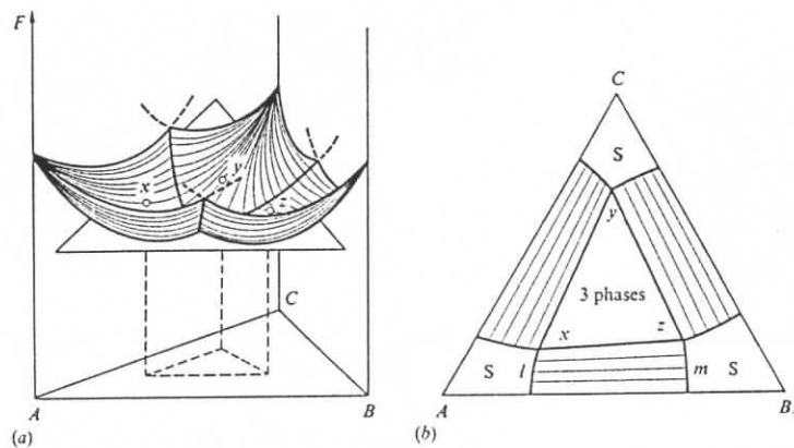
Fig. 5.24. A three-phase equilibrium in the ternary system derived by means of the tangential plane (a) and represented in an isothermal section (b). ( $l - m$ ) = conode.
