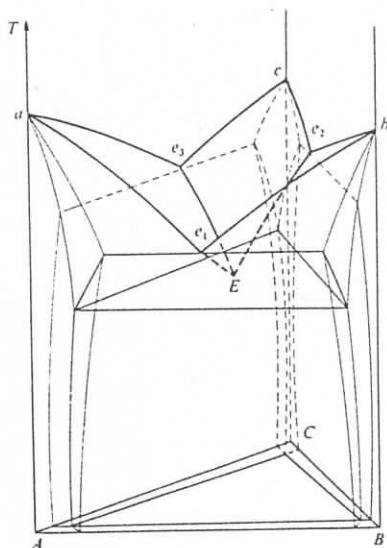
Fig. 5.25. Perspective drawing of a ternary phase diagram with ternary eutectic point  $E$ .
