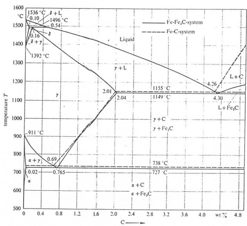
Fig. 6.4. Iron-carbon phase diagram (dotted lines graphite, full lines in equilibrium with  $\text{Fe}_3\text{C}$ ) [5.8].
