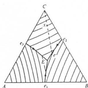
Fig. 5.26. Projection of the liquidus surface of the ternary diagram in fig. 5.25 on to the base.
