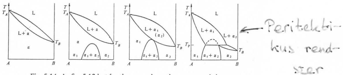
Fig. 5.14. As fig. 5.12 but for the case where the pure metals have widely differing melting points.
