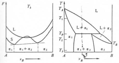
Fig. 5.15. Derivation of a phase diagram with peritectic from  $F^L(v_B, T), F^S(v_B, T)$ .
