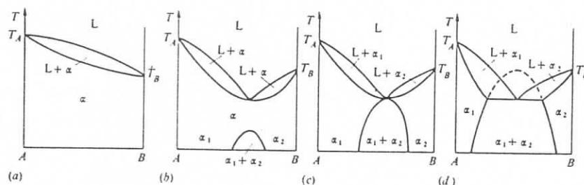
Fig. 5.12. Changes in the phase diagram from (a) to (d) with increasing  $\epsilon$ , i.e. increasing energy of mixing  $E^M > 0$ .
