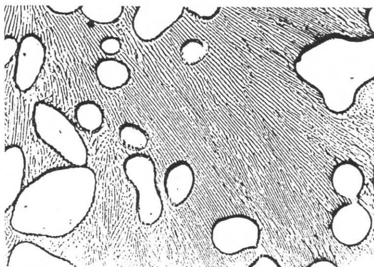
Fig. 4.14. Micrograph of Zn-8% Al showing primary Zn solid solution and eutectic. Cooled in the furnace. 145×.
