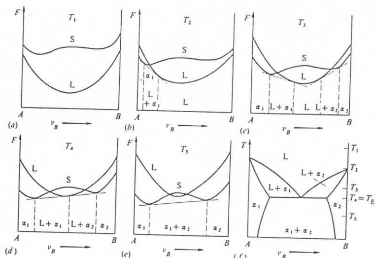
Fig. 5.13. Derivation of a phase diagram with eutectic from the free energy for S and L, dependent on the temperature.
