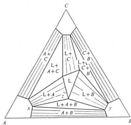
Fig. 5.23. Section through a ternary phase diagram at a temperature above the ternary eutectic temperature but below all the binary  $T_E$ .
