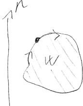
$$\eta = \frac{W}{Q_{\text{fel}}} = \frac{Q_{\text{fel}} - Q_{\text{ee}}}{Q_{\text{fel}}} = 1 - \frac{Q_{\text{ee}}}{Q_{\text{fel}}}$$
