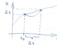
$$v_{\text{átl}}(t_0, \Delta t) = \frac{\Delta x}{\Delta t} = \frac{x(t_0 + \Delta t) - x(t_0)}{\Delta t}$$
