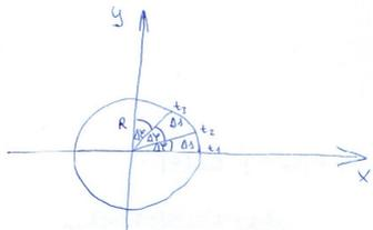
$$\omega(t) = \dot{\varphi}(t) = \omega_0 = \text{állandó}$$
