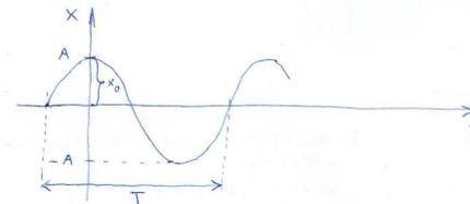
$$A \sin(\omega(t+T)+\varphi) = A \sin(\omega t + \varphi)$$
