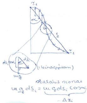
$$W = \int_{z_1}^{z_2} mg ds \approx - \sum_{i=1}^N mg ds_i = -mg \sum_{i=1}^N dz_i = -mg \Delta z = \sum_{i=1}^N mg dz_i$$
