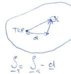
$$\begin{aligned} \Theta_{TKP} &= \sum_i m_i \rho_i^2 \\ \Theta &= \sum_i m_i \rho_i'^2 = \sum_i m_i (\rho_i - a)^2 = \sum_i m_i (\rho_i^2 - 2 \rho_i a + a^2) = \\ &= \sum_i m_i \rho_i^2 - 2 \sum_i m_i \rho_i a + \sum_i m_i a^2 = \\ &= \Theta_{TKP} - 2 \underbrace{\left( \sum_i m_i \rho_i \right)}_0 a + M a^2 = \\ &= \boxed{\Theta_{TKP} + M a^2} \end{aligned}$$
