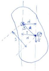
$$\begin{aligned} \vec{G} &= M \cdot g \\ M_2 &= 0 \\ M &= \Theta \cdot \beta \\ M &= -mgs \sin \varphi \\ \varphi + \frac{mgs}{\Theta} \sin \varphi &= 0 \end{aligned}$$
