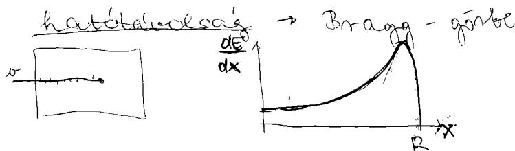
$$R = \int_0^R dx = \int_{E_0}^0 \frac{dx}{dE} dE = - \int_{E_0}^0 \frac{1}{\frac{dE}{dx}} dE = \int_{E_0}^0 \frac{dE}{\sigma_{st}} = \int_{E_0}^0 \frac{dE}{(\dots) \frac{Z^2 A}{E}} =$$
