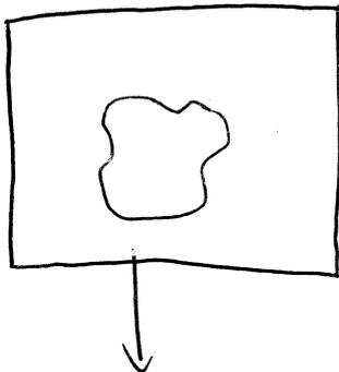
$$F_{\text{fel}} = \oint \hat{\sigma} dA = \int_V (\text{div } \hat{\sigma}) dV = - \int_V \rho \cdot g dV = - \rho \cdot g \cdot V_{\text{(test)}}$$
