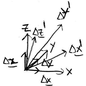
$$\underline{\Delta x} = (\Delta x, 0, 0), \quad \underline{\Delta y} = (0, \Delta y, 0), \quad \underline{\Delta z} = (0, 0, \Delta z)$$
