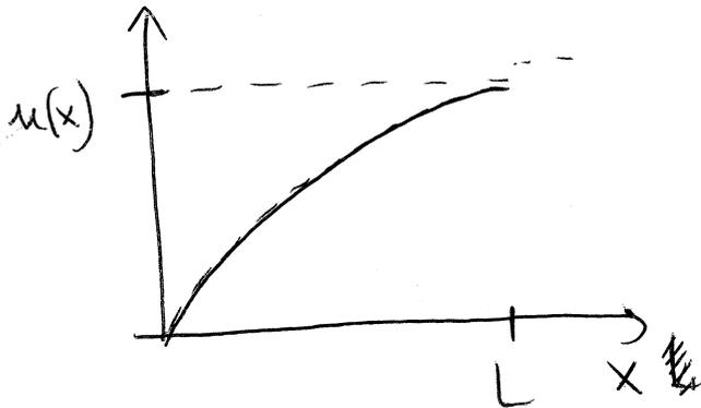
$$u(L) = \frac{1}{2} \frac{L}{EA} \underbrace{\rho g LA}_{V_{\text{negd}} \cdot \rho g} = \frac{1}{2} \frac{mg}{EA} L$$
